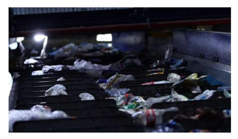
Carbon black = <u>not</u> detectable by NIR sorting equipment (near- infrared spectostropy)
